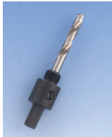
1/4" ARBOR DRILL BIT Used for holesaws, they have a 5/8" thread to suit holesaws 14-30mm and 31-200mm with an 11mm chuck. CODE: ARBOR1 ARBOR2 CHUCK: 11mm 11mm SIZE: 14-30mm 31-200mm
