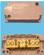
METER LINK 165A Rated at 165A, comes in a white colour for easy labelling of active and neutral, maximum cable size 50mm. CODE: ML165/7 ML165/13 7 HOLE 13 HOLE
